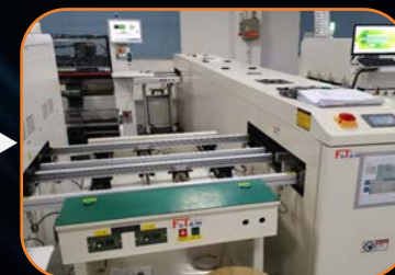
Fully - automatic Conveyor Belt
