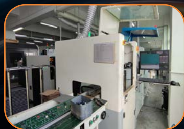
Automatic brushing of three - proof paint
