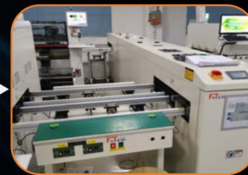
Fully - automatic Conveyor Belt
