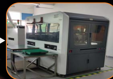
Automatic Screw - Tightening
